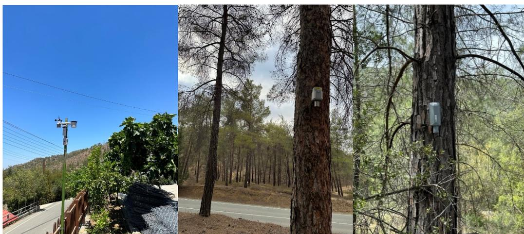
**Figure 10:** Installed sensors (Weather Station left, EM500 centre, SenseCAP S2103 right).
