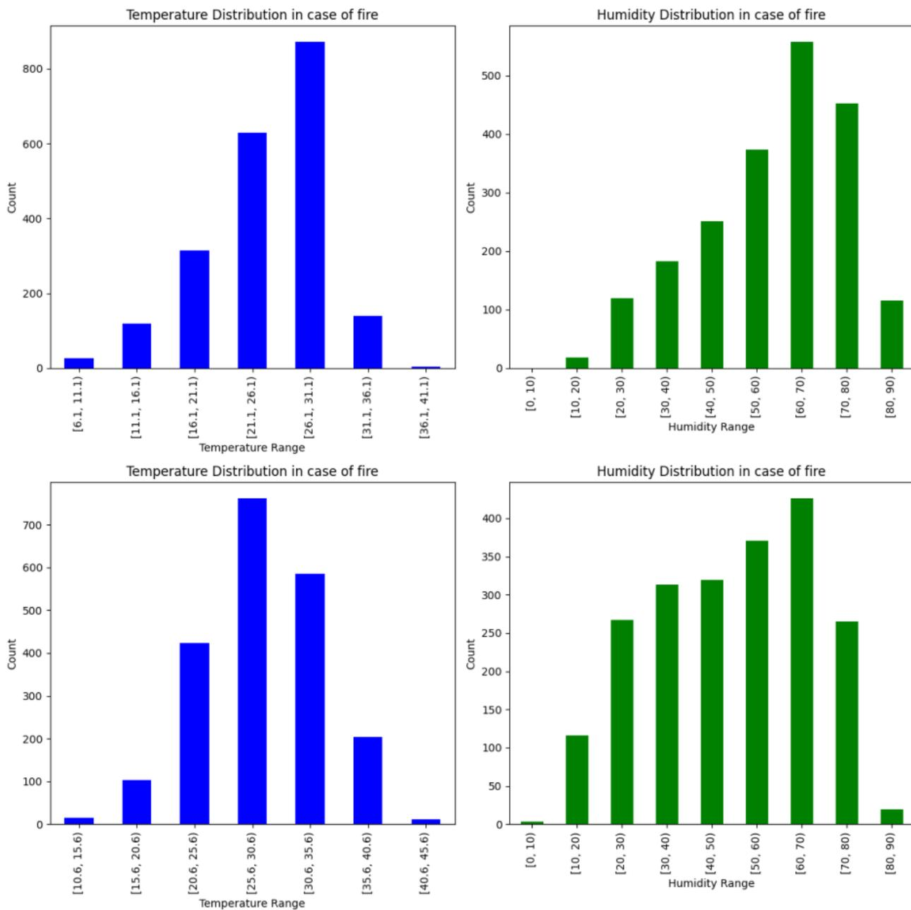
**Figure 7:** Temperature and Humidity distribution in case of fire
